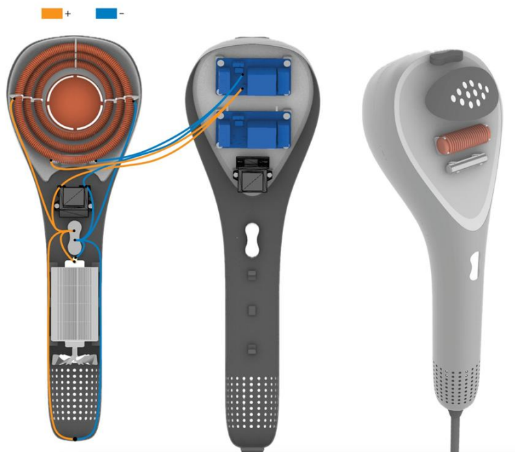
Figure 8 Electrical wire layout for the hair dryer.
