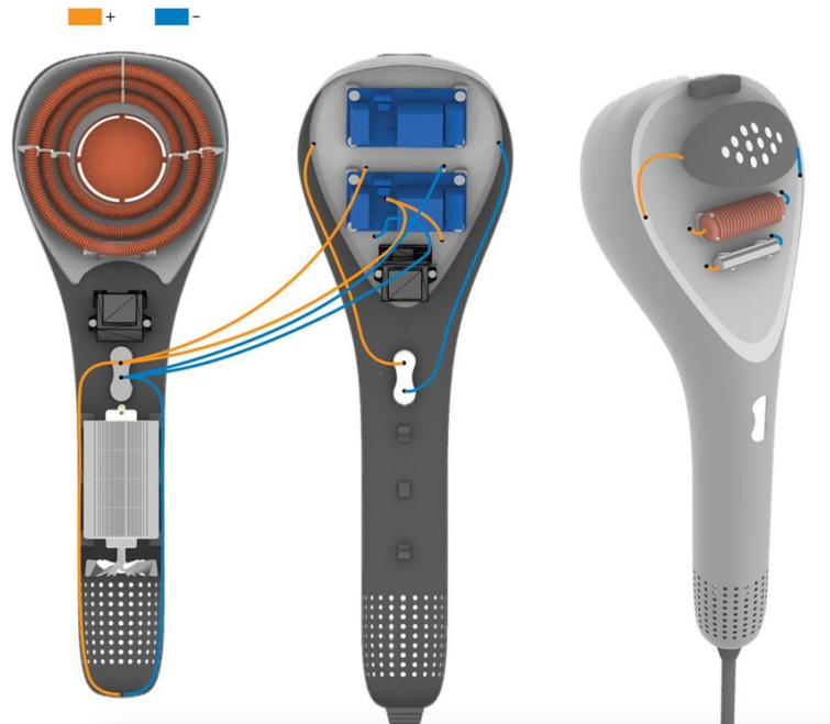
Figure 9 Electrical wire layout for steam iron.
