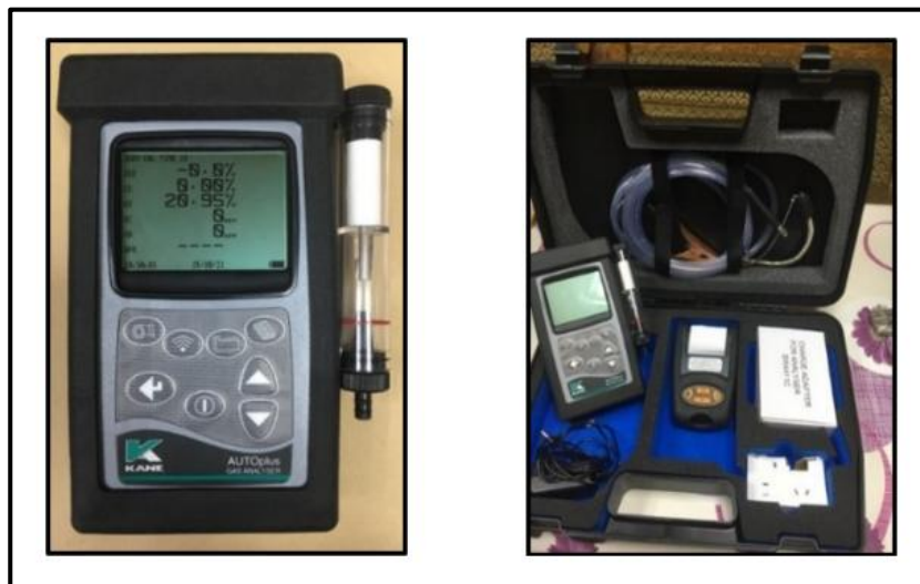
Figure 1. KANE AUTO 5-1 Portable Car Emission Analyzer OIML Class 1-5 gases [15].
