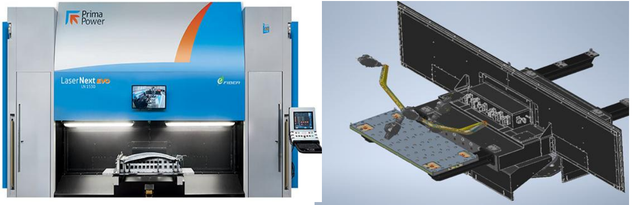
Figure 3. Prima Power Next laser cutting equipment: a – front view; b – workpiece orientation and fixation device
