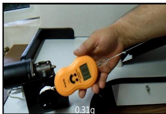
Figure 12 (b). Result of the experiment an exponential hoist (muffle) with 2 pulleys.
