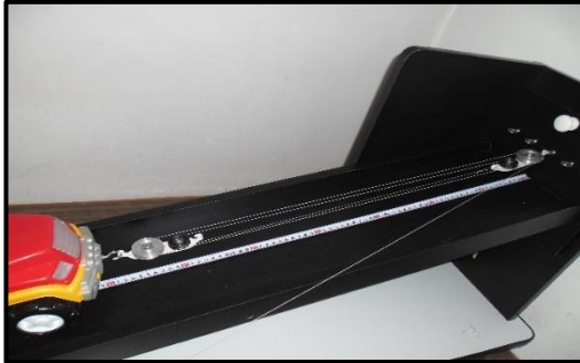
Figure 14 (a). Experiment a factorial hoist (muffle) with 4 pulleys.
