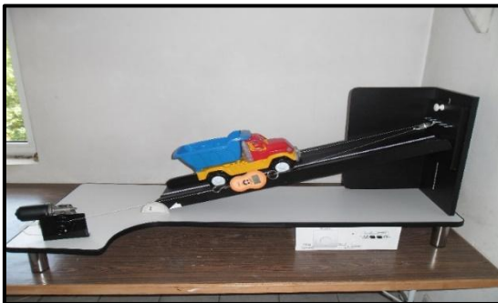
Figure 8. Device for towing and embarking rough terrain vehicles.
