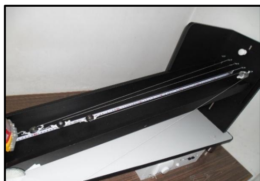
Figure 13 (a). Experiment with an exponential hoist (muffle) with 3 pulleys.
