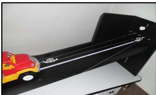
Figure 11 (a). Experiment with a mobile pulley.
