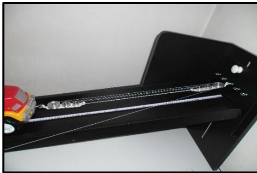
Figure 15 (a). Experiment a factorial hoist (muffle) with 6 pulleys.
