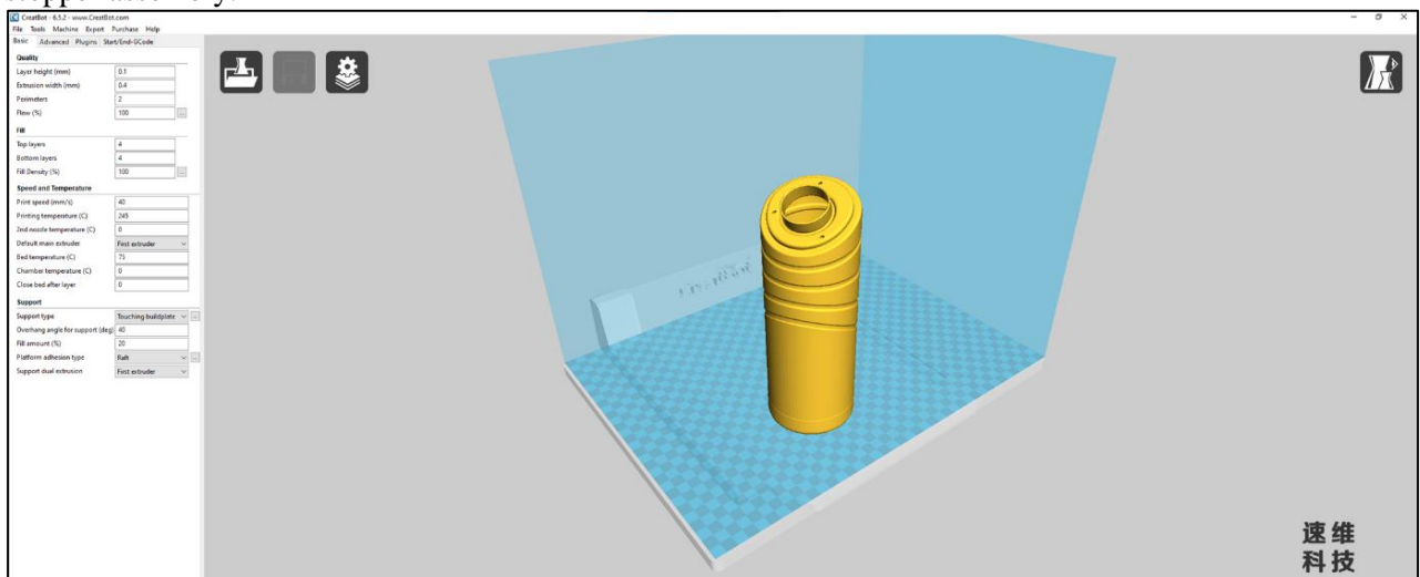
Figure 8. Print screen of the 3dimensional model imported in Slicer software
