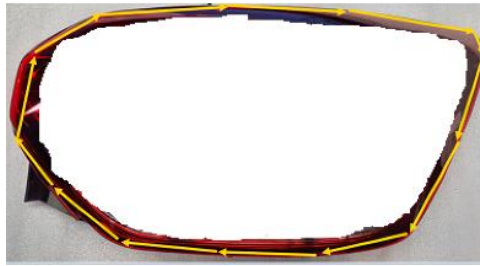
Figure 7. Part contour and direction of welding
