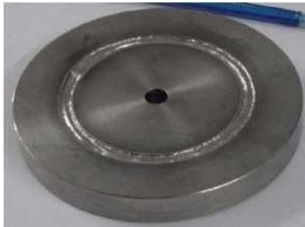
Figure 5. Circular weld -Ti-6Al-4V
