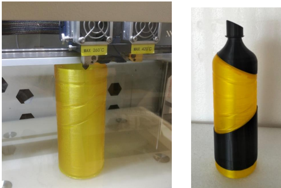
Figure 9. 3 D printed model of the 1 liter packaging, scale 1:1
