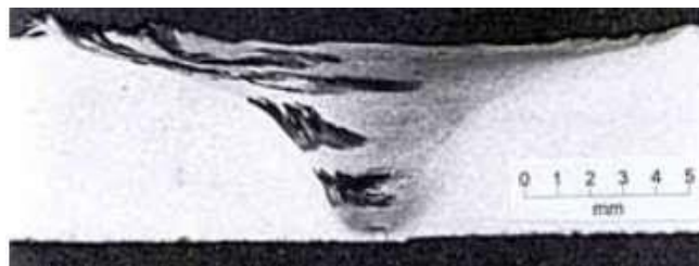
Figure 3. A quality FSW joint in 6.35 mm thick Ti-6Al-4V (photo taken from IWI)[11]
