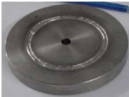
Figure 5. Circular weld -Ti-6Al-4V
