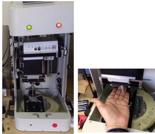
Figure 1. CETR test bench adapted for skin tribology
